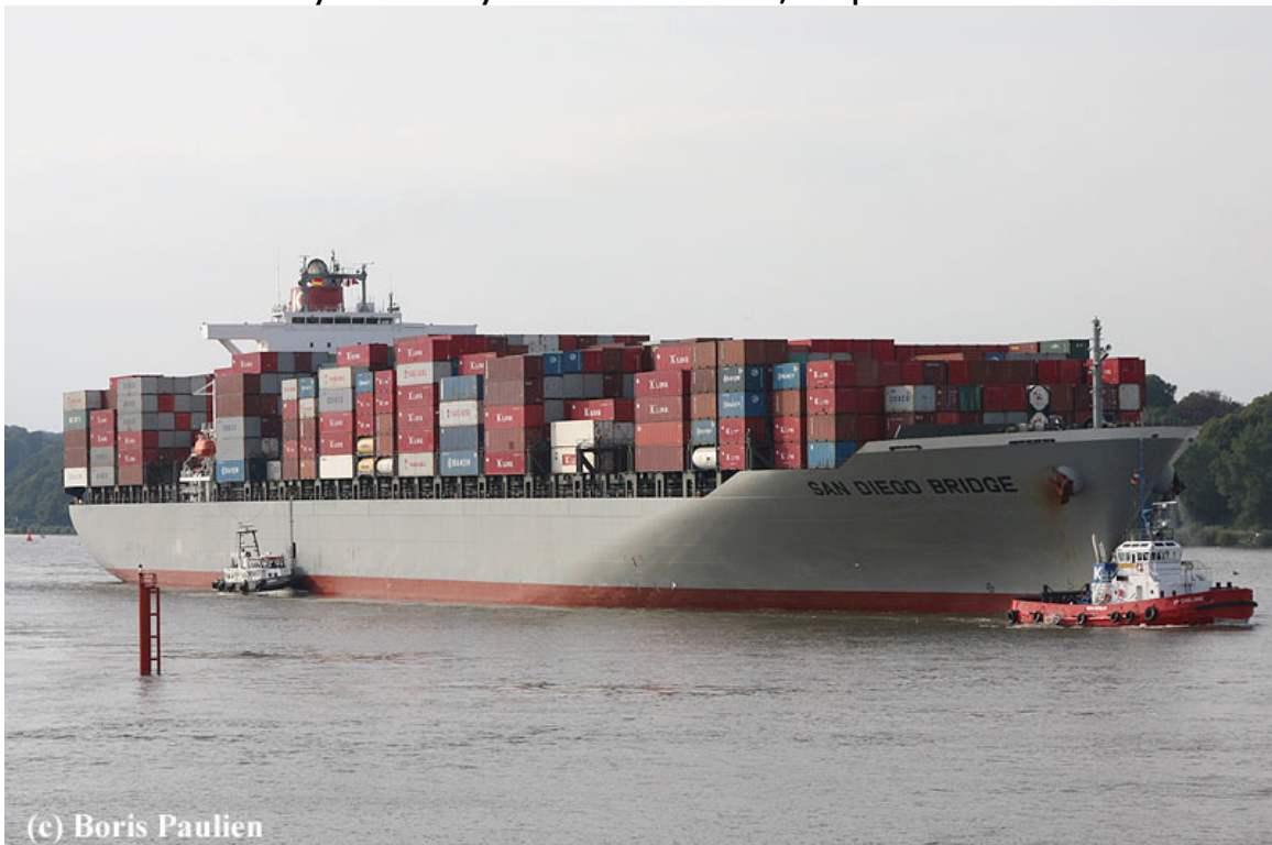
...later, the ship comes into Hamburg. At 6,350 teu, she is rather a small ship to trade in a Far East-Europe mainline service.
