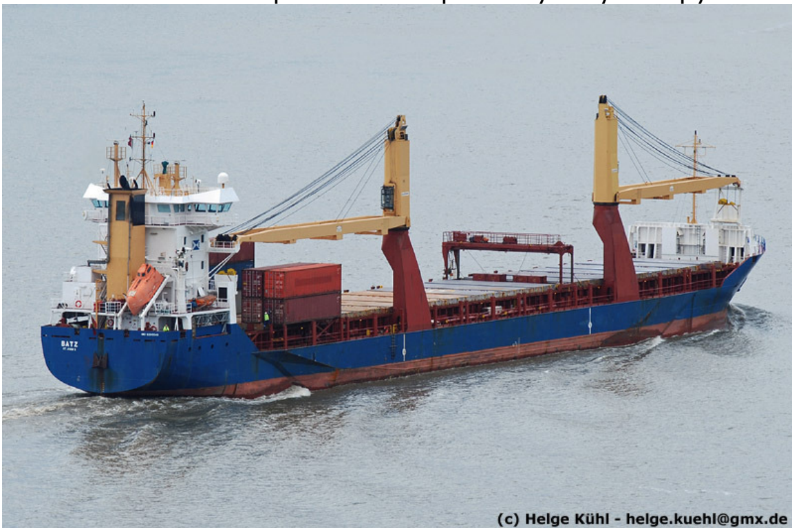
The 665 teu mpp ship BATZ, since renamed SE DIONYSUS, is one of almost 50 units of the Damen Combi-Freighter 10200 design.
