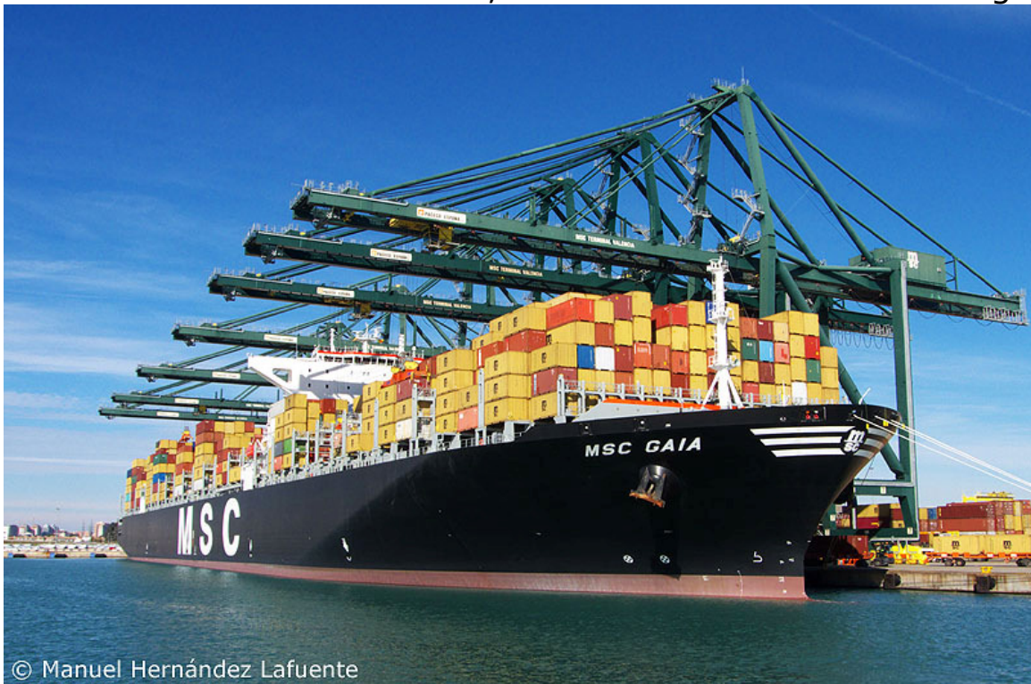
Another jumbo, the Samsung-built 14,000 teu ship MSC GAIA, is handled at Valencia, MSC's west Mediterranean hub port.
