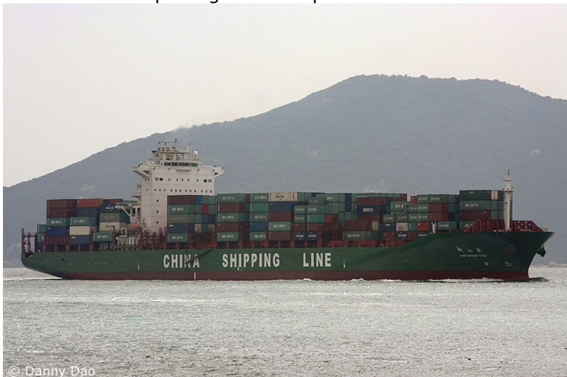
XIN SHAN TOU was built in 2005 by Dalian New Shipyard. Here, the 4,250 teu near-panamax vessel comes into Hong Kong.
