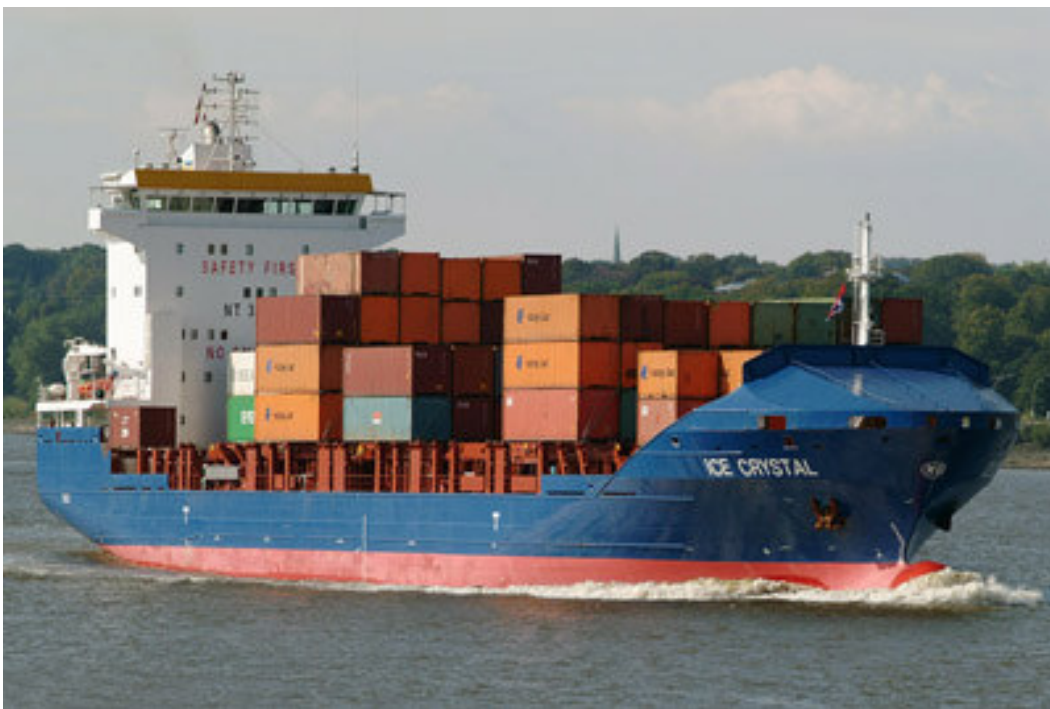
The Mawei-built 700 teu feeder ICE CRYSTAL arrives at Hamburg with a load of Hapag-Lloyd boxes.
