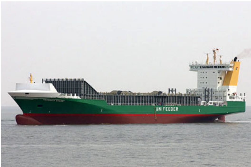
HEINRICH EHLER is the first ship of Sietas's new type178 semi open top design. Here runs trials on the river Elbe.
